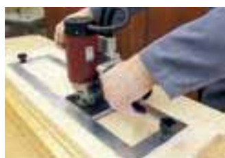
Milling jig for Minispot patching rods
