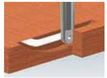
Glue application on the sides
